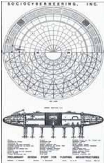
From the tops of these structures, a cylindrical concrete conduit extends 150 feet above the ocean surface. At surface level, it is encircled by a floating dock system, which rises and falls with the tides and accommodates both surface and submersible craft.
